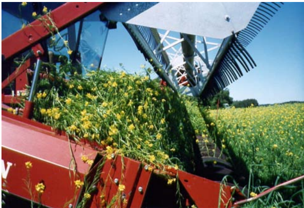
Figure 1. Weed Buildup on the Unmodified Table with Canvases Removed.
